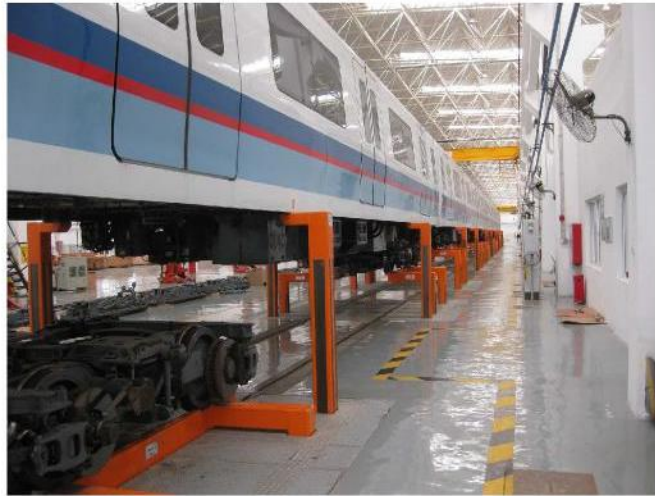
Lifting systems for rail-bound vehicles as per EN 1493
