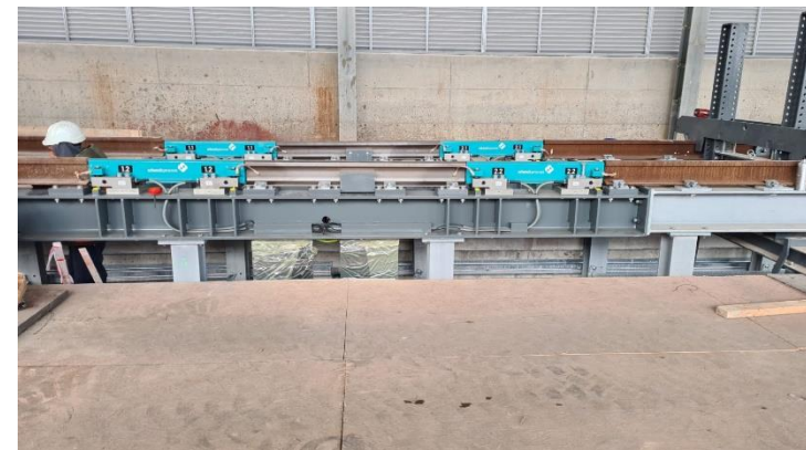
Integrated weighing system in a high-precision measuring track
