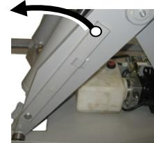
For all further transaction, the mounted-on maintenance support have to be put in.
