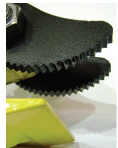
***CH with serrated jaw which can only be used for single plates, NOT bundles.
