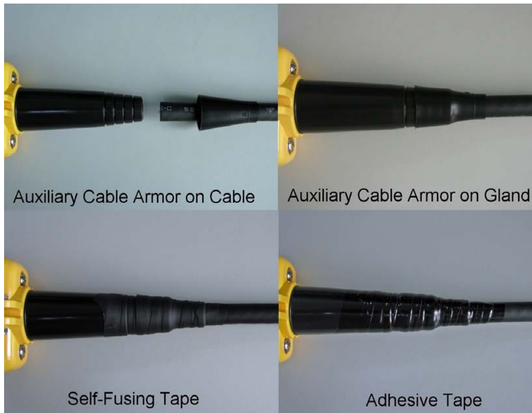
Figure 2: Auxiliary Cable Armor Installation
