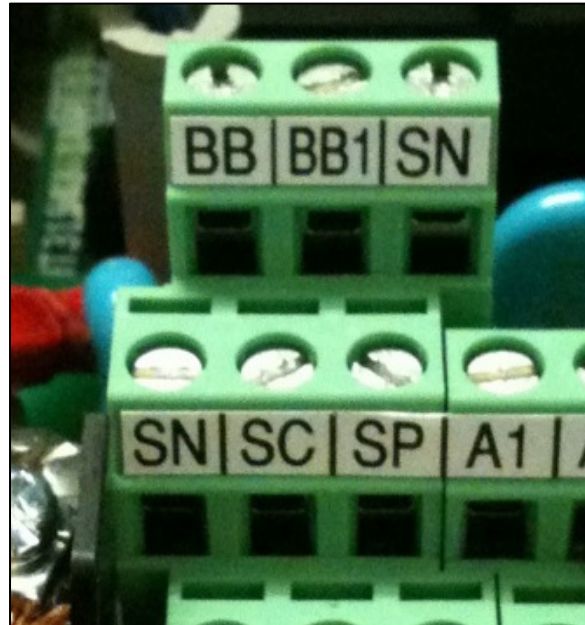
Figure 4: Safe-Off terminals (BB, BB1, SN)
